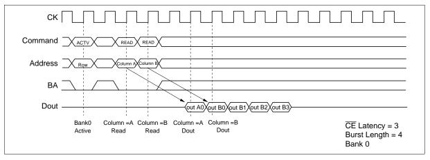
**2.** Same bank, different ROW address: When the ROW address changes on same bank, consecutive read commands cannot be executed; it is necessary to separate the two read commands with a precharge command and a bank-active command.
