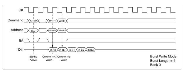
WRITE to WRITE Command Interval (same ROW address in same bank)
