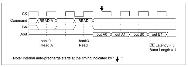
Read with Auto Precharge to Read Command Interval (Different bank)
