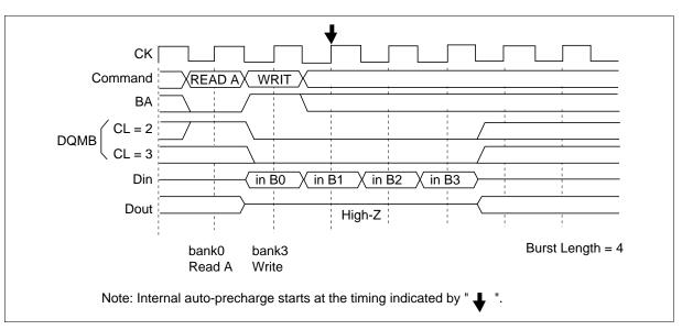
Read with Auto Precharge to Write Command Interval (Different bank)
