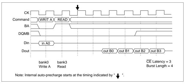
Write with Auto Precharge to Read Command Interval (Different bank)
